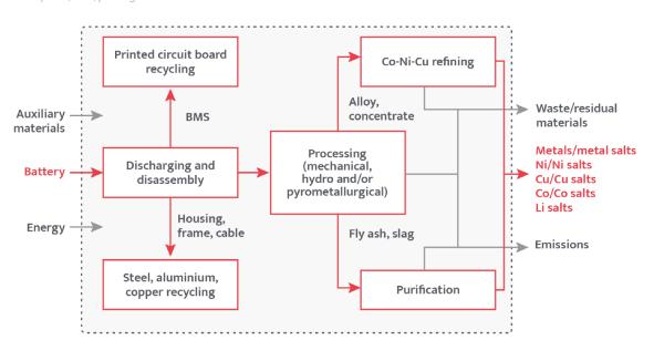
Initially, waste batteries are collected, sorted, discharged and disassembled (Figure 2). This is followed by mechanical crushing, drying, sorting sieving and pyrolysis to 700°C to remove any remaining electrolyte and potentially hazardous to health fluorine-containing components (Figure 3). The resulting material is what is referred to in the battery recycling industry as 'black mass'.
